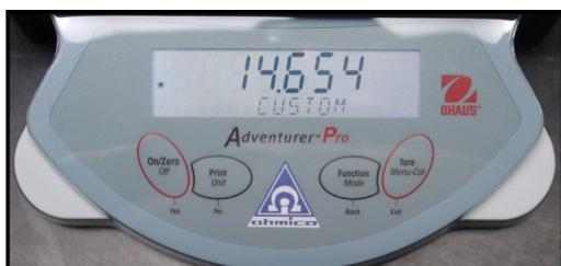
UPM-DT Series Ultrasound Power Meters feature a high contrast alphanumeric LCD display. Membrane "touch buttons" enable quick setup, automatic zero, selection of units for the power reading (grams or Watts "custom"), and printer control.
